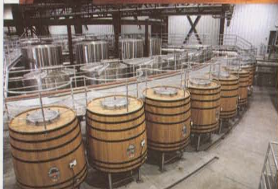
"We can store three vintages at a time in here," remarks Don Carano. (above) French-built oak Fermentation tanks form the final ring of the Mountain Estate Winery's radial plan.
